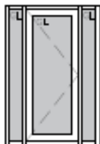
A-4 ALUMINUM ENTRANCE SYSTEM ALUM. DOOR TEMPERED THERMAL UNIT ALUM. FRAME CLEAR ANODIZED
